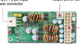
Main / Mini-Fit 20 pin output power connector
