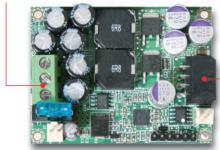
12V / Mini-Fit 8 pin output power connector
