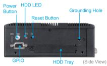
The CHUMPI-5390 is powered by Intel® Atom™ quad-core processor. Despite its fan-less and cable-less design, the system can support wide temperature ranging from -30°C ~ 70°C degrees. By utilizing the low power technology, CHUMPI-5390 is an ideal platform for factory automation and transportation applications.
