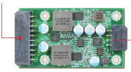
12V / Mini-Fit 8 pin input power connector
